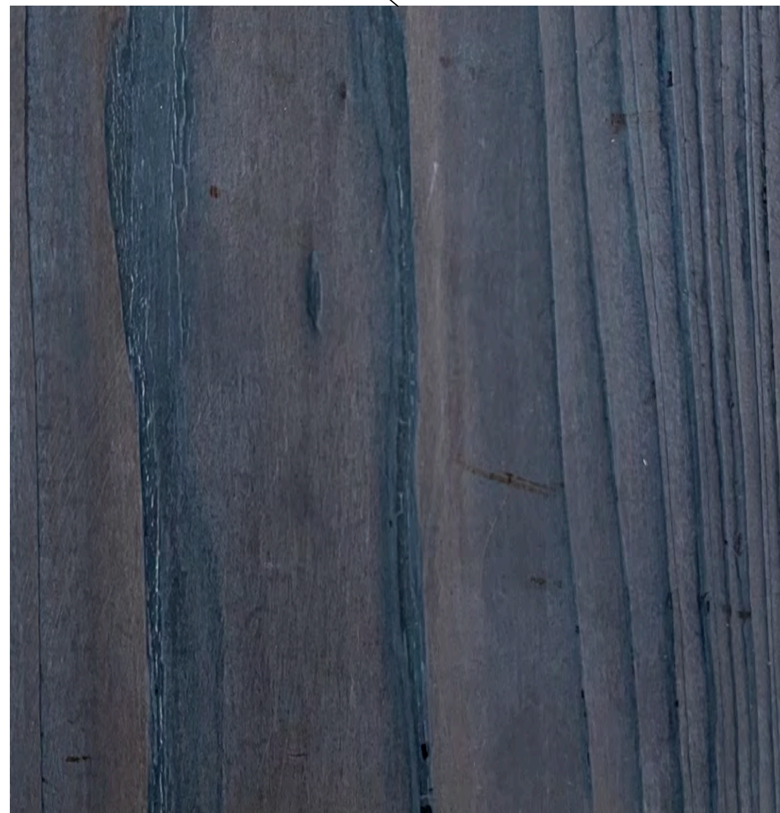
EXTERIOR SIDING DELTA MILLWORKS ACCOYA - SB - BURNED AND BRUSHED - 1x6 WHITE WASH APPLIED BY CONTRACTOR
