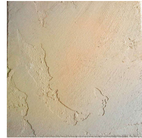
ROUGH STUCCO FINISH
