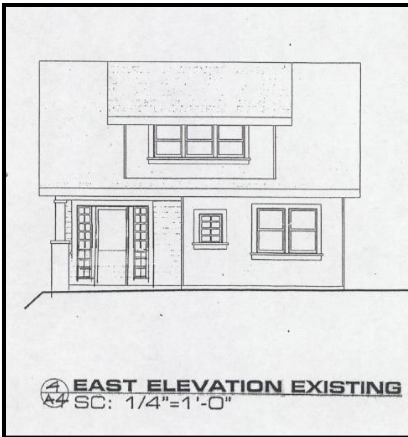
Figure 1: 2008 elevation of the original front porch pier, and the original window glazing on the first floor and dormer windows.
