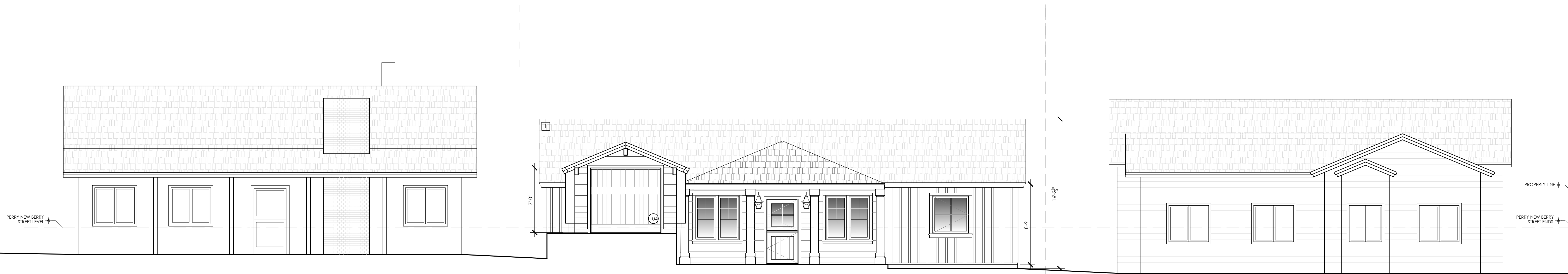
2 EAST ELEVATION PROPOSED STREETSCAPE ELEVATION SCALE: 3/16" = 1'-0"
