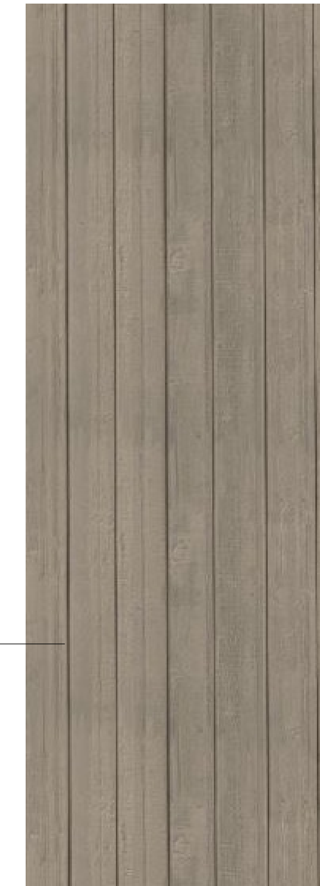
VERTICAL CEDAR SIDING (STAINED)
