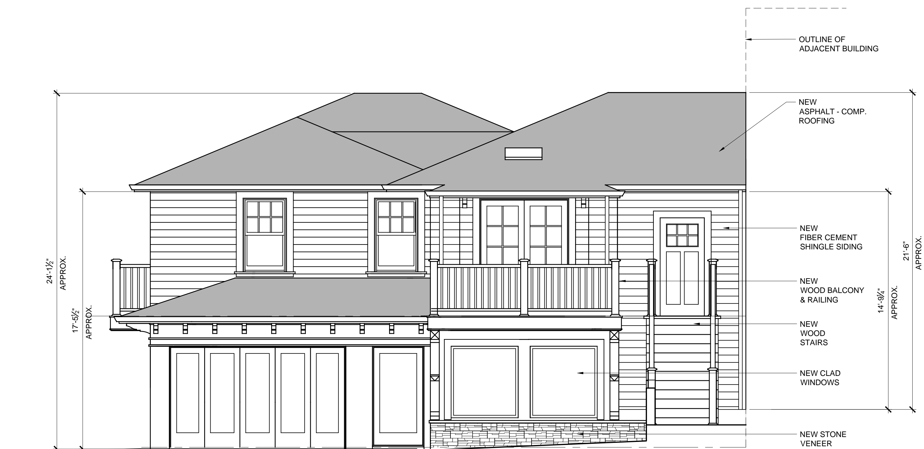
1 FRONT EXTERIOR ELEVATION SCALE: 1/4" = 1'-0"
