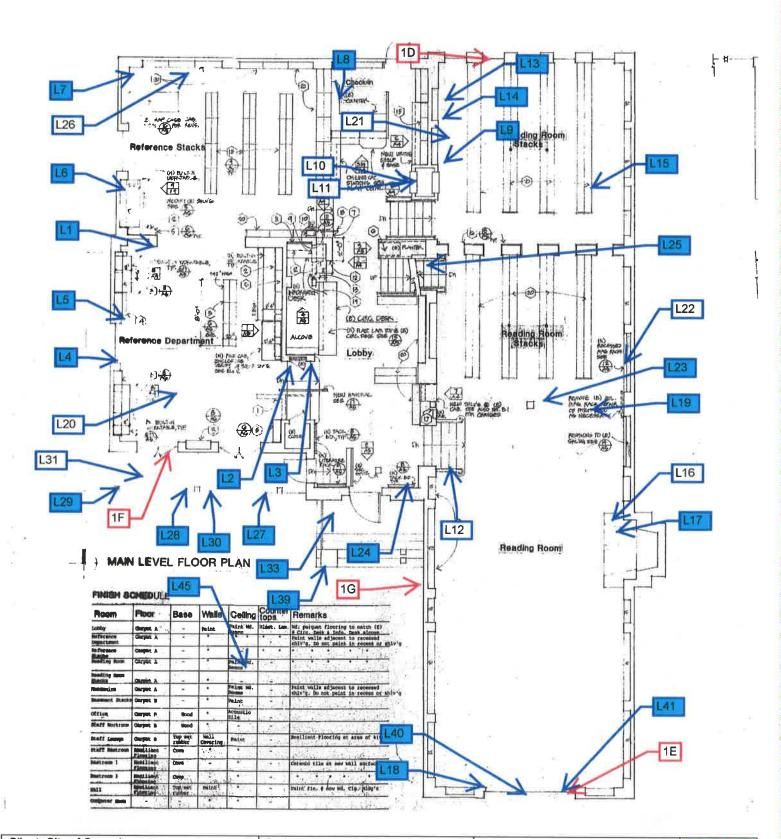
Client: City of Carmel Project Name: ACM/Pb Reno Location: Harris Library Floor: Upstairs Project No. 22207.0 – T1 Date: 6/2/22 Key: Asbestos sample Lead sample Positive material
