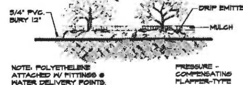
**NOTE:** POLYETHYLENE ATTACHED W/ FITTINGS @ WATER DELIVERY POINTS.
