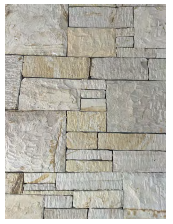
CARMEL STONE @ ENTRY AND CHIMNEY
