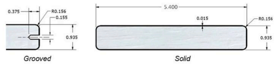
FIGURE 3—FIBERON® CONCORDIA™ ASTIR, CONCORDIA™ HORIZON® AND CONCORDIA™ SYMMETRY® CROSS-SECTIONS
