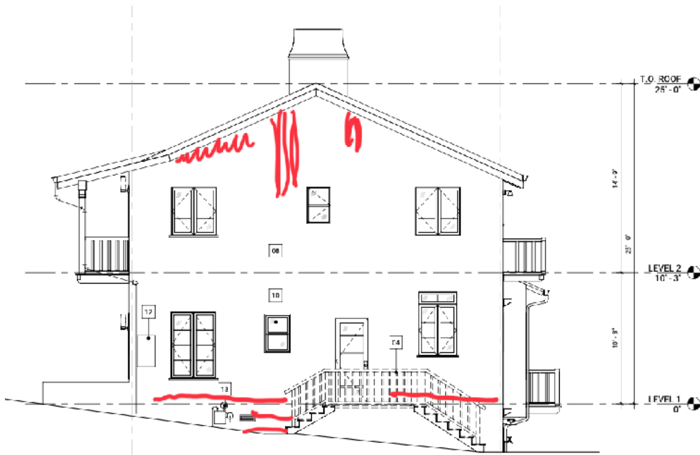
② DEMOLITION BUILDING ELEVATION - NORTH 1/4" = 1'-0"
