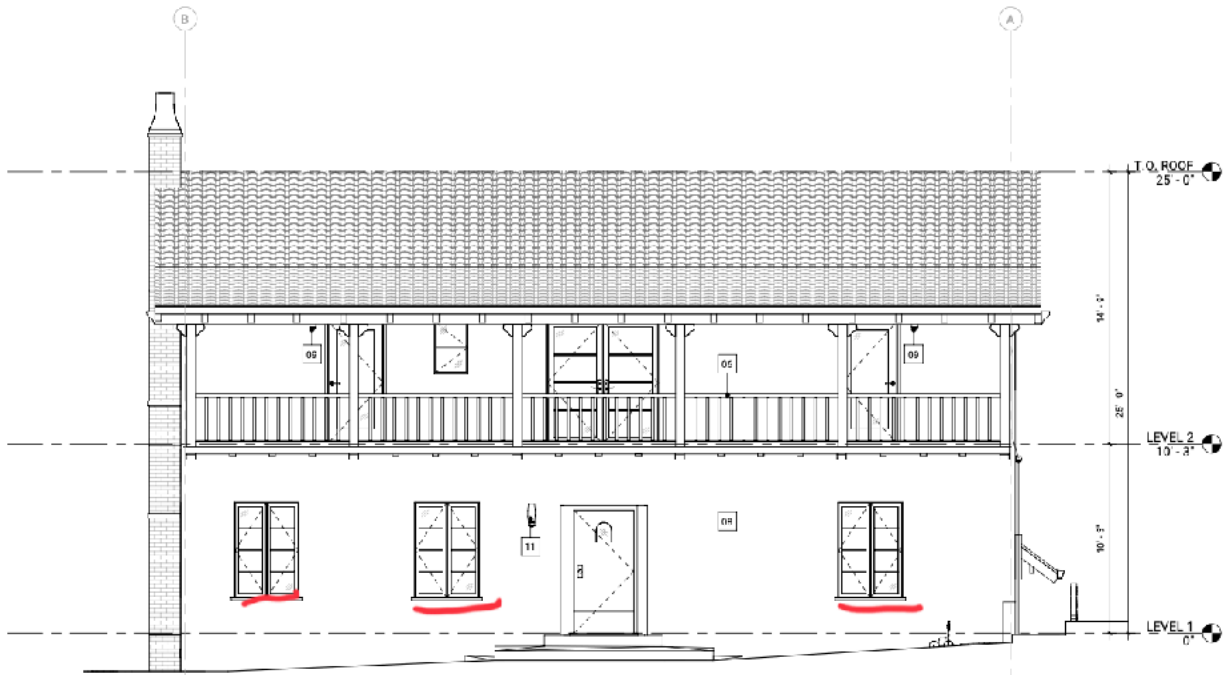
① DEMOLITION BUILDING ELEVATION - EAST 1/4" = 1'-0"
