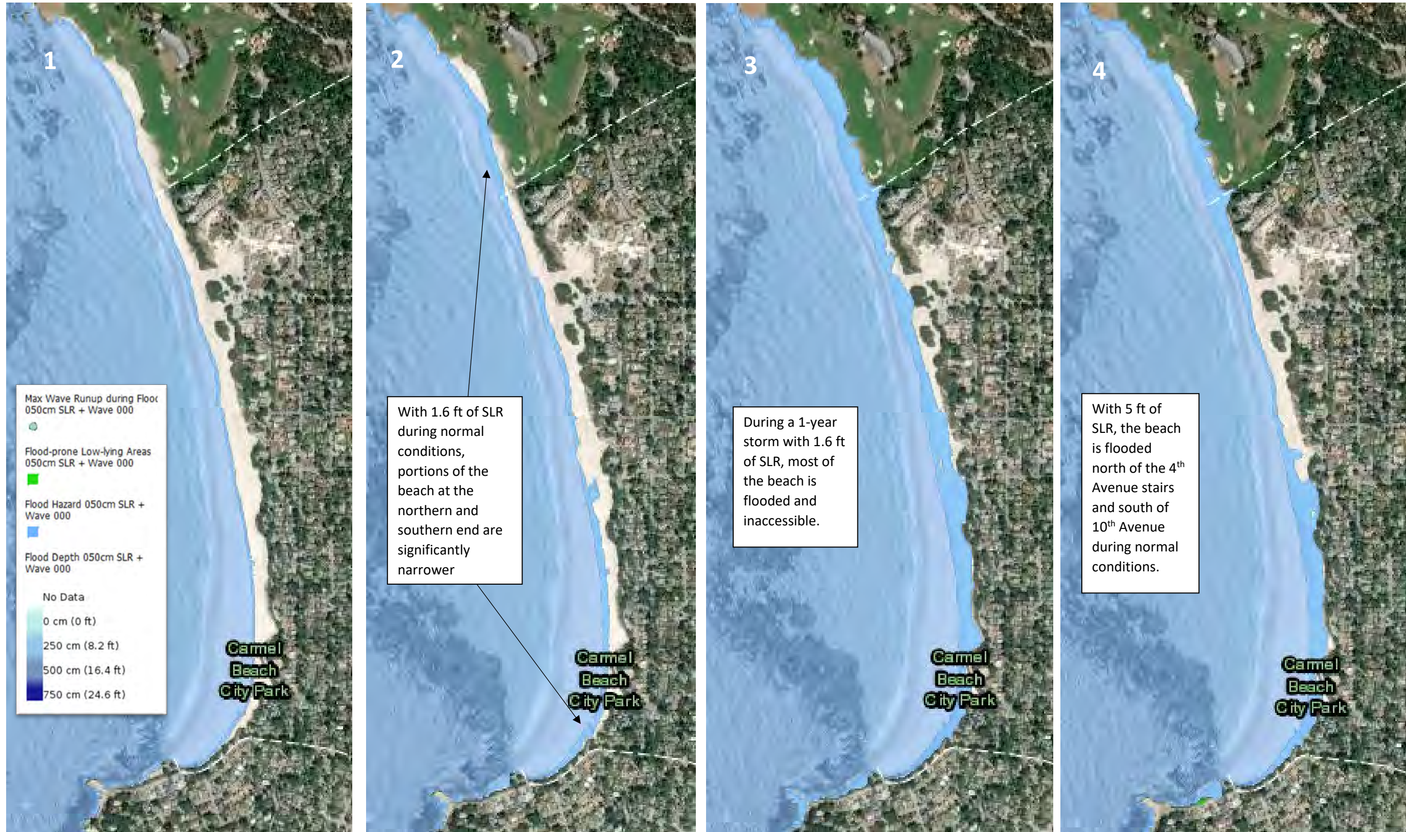
Figure 2: Comparison of Carmel Beach maximum wave run-up during: 1) current conditions, 2) with 1.6 ft of sea level rise (SLR) and no storm, 3) 1.6 ft of SLR and 1-year storm, and 4) 5 ft of SLR and no storm.
