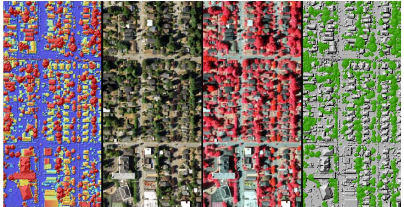
Three different ways to measure tree canopy from left to right: LiDAR, aerial photography, and color infrared, with Seattle's final LiDAR-based tree canopy result mapped on the far right. Source: City of Seattle.
