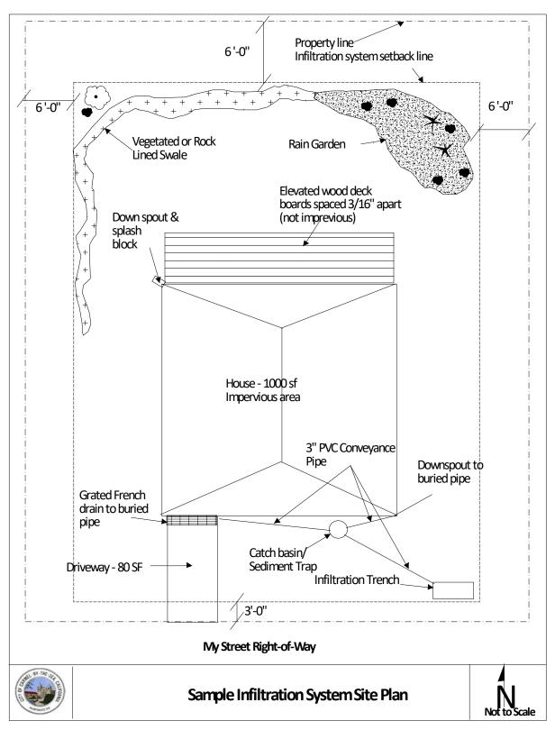
This Sample Infiltration System Site Plan provides an example of a complete drainage system site plan. It illustrates a variety of systems and components. Not all components are used in every system. Your system and plans may vary however must provide equivalent detail for your project
