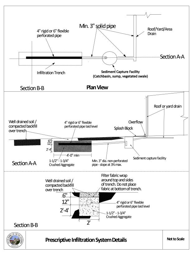
These Prescriptive Infiltration System Details specifically apply to the prescriptive path systems addressed on Page 2 of this document. Prescriptive systems are required to contain these features. Engineered systems may differ.
