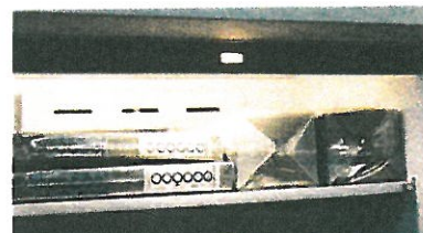
Figure 3. Do not cover air vents, such as the slotted ones in the back of this freezer, with boxes.
