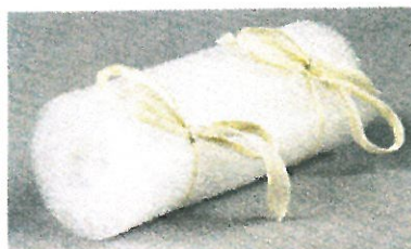
Figure 3. Roll small pieces of Ethafoam™ and tie with twill tape and use to fill voids in boxes.
