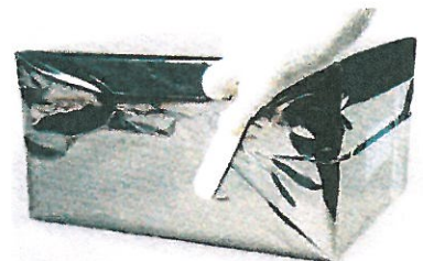
Figure 5. A bone folder is being used to “burnish” tape to ensure it adheres to the package.
