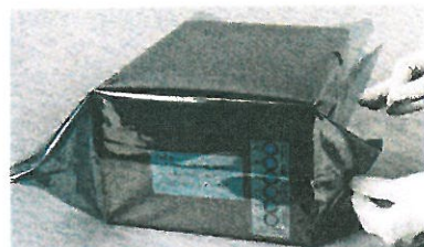
Figure 4. Inner bag being wrapped. Excess material and flaps are tightly secured with tape along the sides.
