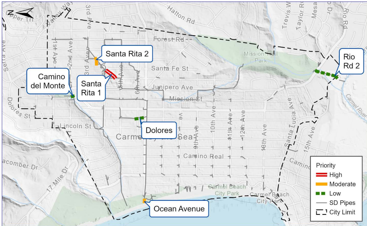
Figure 4-4: Observed Condition Issues
