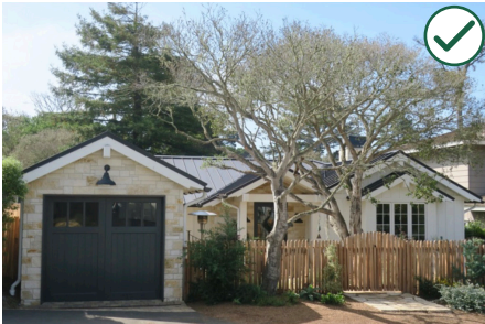
Only a one-story building is appropriate for a garage that is permitted to encroach into the front setback.
