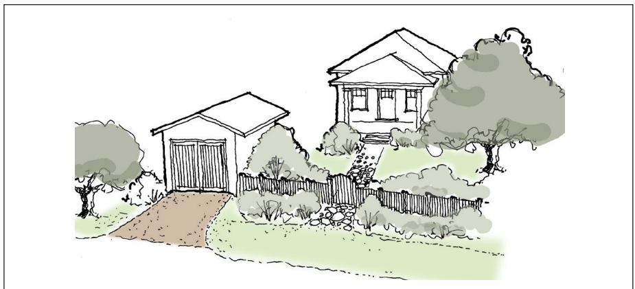
In this sketch, a garage is permitted to encroach into the front setback.
