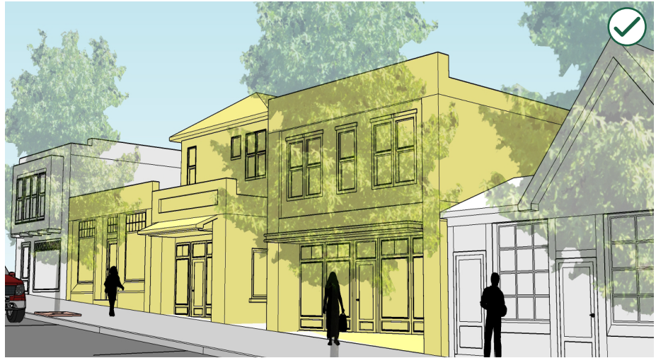
In this conceptual sketch, a new building is represented in yellow. It is organized in three modules that reflect traditional lot widths. Wall heights vary at the sidewalk edge and some upper stories are set back to reduce perceived size.
