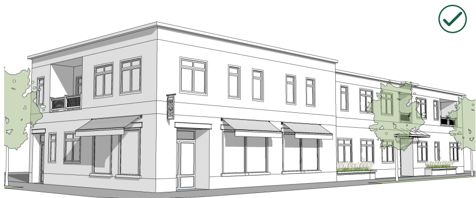
A flat roof is an appropriate form for a Mixed-use Multifamily building.
